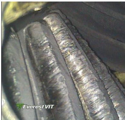
Figure 6 - Article 1 input gear after catastrophic failure
