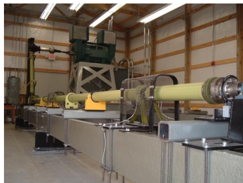
Figure 1 - USC AH-64 Tail Rotor Drive Train test stand
