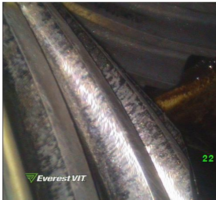
Figure 8 - Article 3 input gear after gearbox core temperature instability
