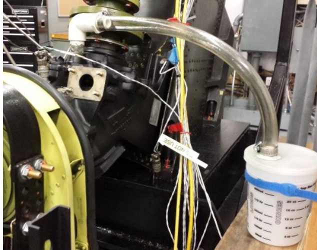
Figure 4.2 Breather port adapter setup
