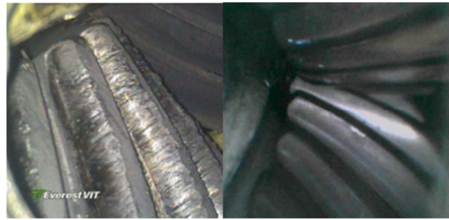
Figure 7. A comparison, from a previous experiment, of worn gear teeth (left) to healthy teeth (right)
