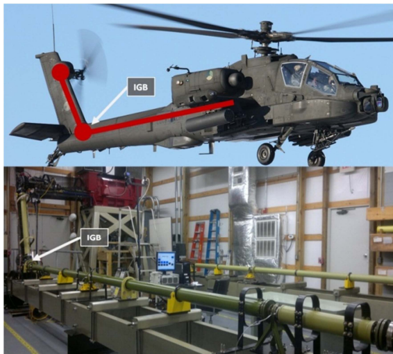
Figure 1. Comparison of USC test stand to actual aircraft
