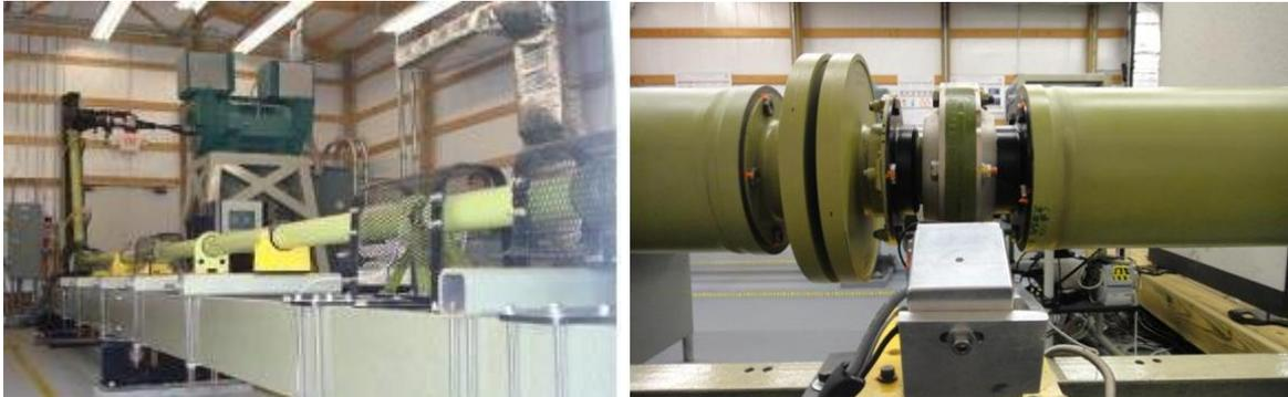
**Figure 2: Tail Rotor Drive Train test stand. ADVISER monitoring the aft hanger bearing**
