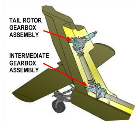
**Figure 2 - AH-64 tail rotor and intermediate gearbox assembly location**
