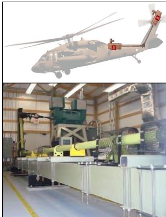
Fig. 2. USC Tail Rotor Drive Train (TRDT) test stand.
