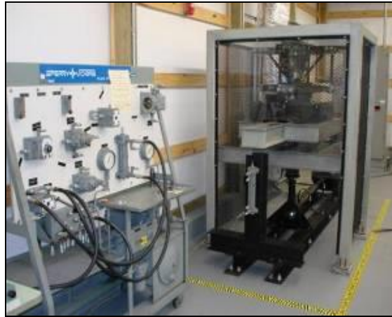
Fig. 3. USC Main-Rotor Swash-plate (MRSP) assembly test stand.
