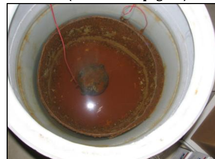
Figure 3 New steel anode ring and rust build up after a 3-month period of electrolysis
