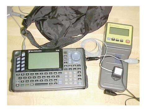
The CBL is a portable data acquisition unit that connects to calculators for easy readout of data. A "single-axis, low-g" accelerometer attaches to the CBL to measure forces that give rise to accelerations between 0 and 5 times the acceleration due to gravity (5 g's). The CBL and accelerometer fit in a waist pack for safe transport on the midway rides.
