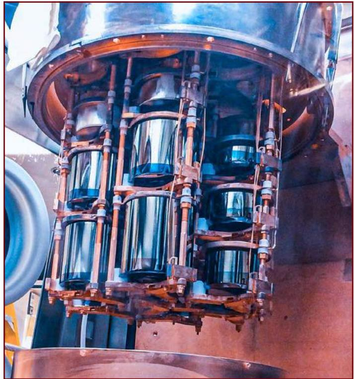
*An inside look at the Germanium detectors used in the MAJORANA Demonstrator. The larger detectors in the foreground are newly installed and are being performance tested for future use in the LEGEND experiment.*
