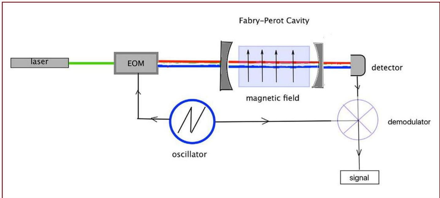
**Figure 2:** A highly over-simplified view of FPAS. Light from the laser passes through an electro-optical modulator (EOM) that and then enters the Fabre-Perot cavity where photons are converted to ALPs in the magnetic field (indicated by the black arrows). The intensity of the light that emerges from the cavity has an intensity modulated at the driving frequency of the EOM.
