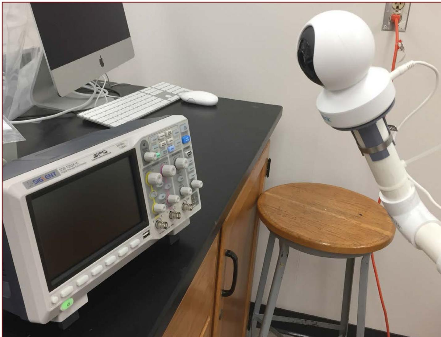
*Prof. Rosenfeld's alter ego. Battery powered clones of this device will allow remote students to converse with their lab partner and to have a close-up real-time view of the apparatus and instruments.*
