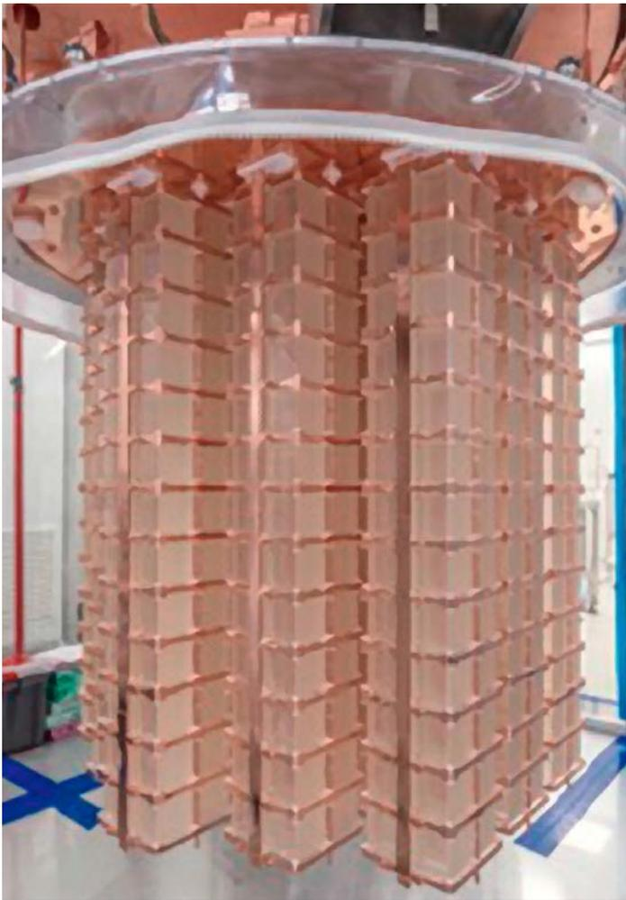
*Tellurium crystals that make up the heart of the CUORE experiment at the Laboratori Nazionali del Gran Sasso in Assergi, Italy.*
