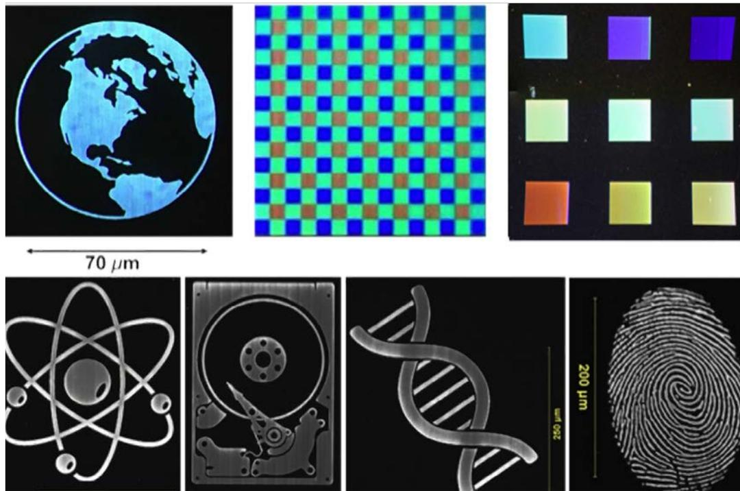
**Figure 2:** Examples of optical diffraction from nanoparticles assembled into nanoscale gratings that are patterned at the macroscale (>50 μm) into a variety of recognizable images. For the multi-colored square patterns, each square has a different period grating diffracting a different color in the vertical direction.
