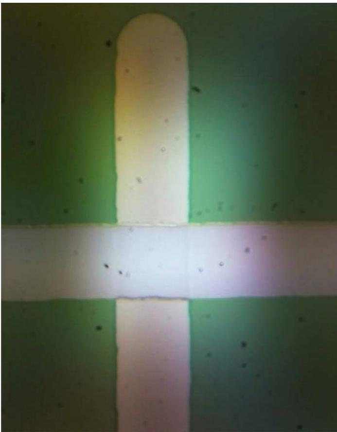
Optical microscopy image of a cross-bar array memristor.
