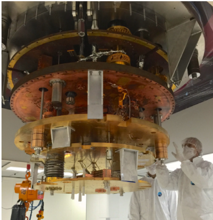
CUORE researchers working on the bottom of the CUORE Dilution Refrigerator at LNGS.
