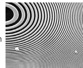
Zone plate x-ray "lens" Outer ring spacing ~35 nm
