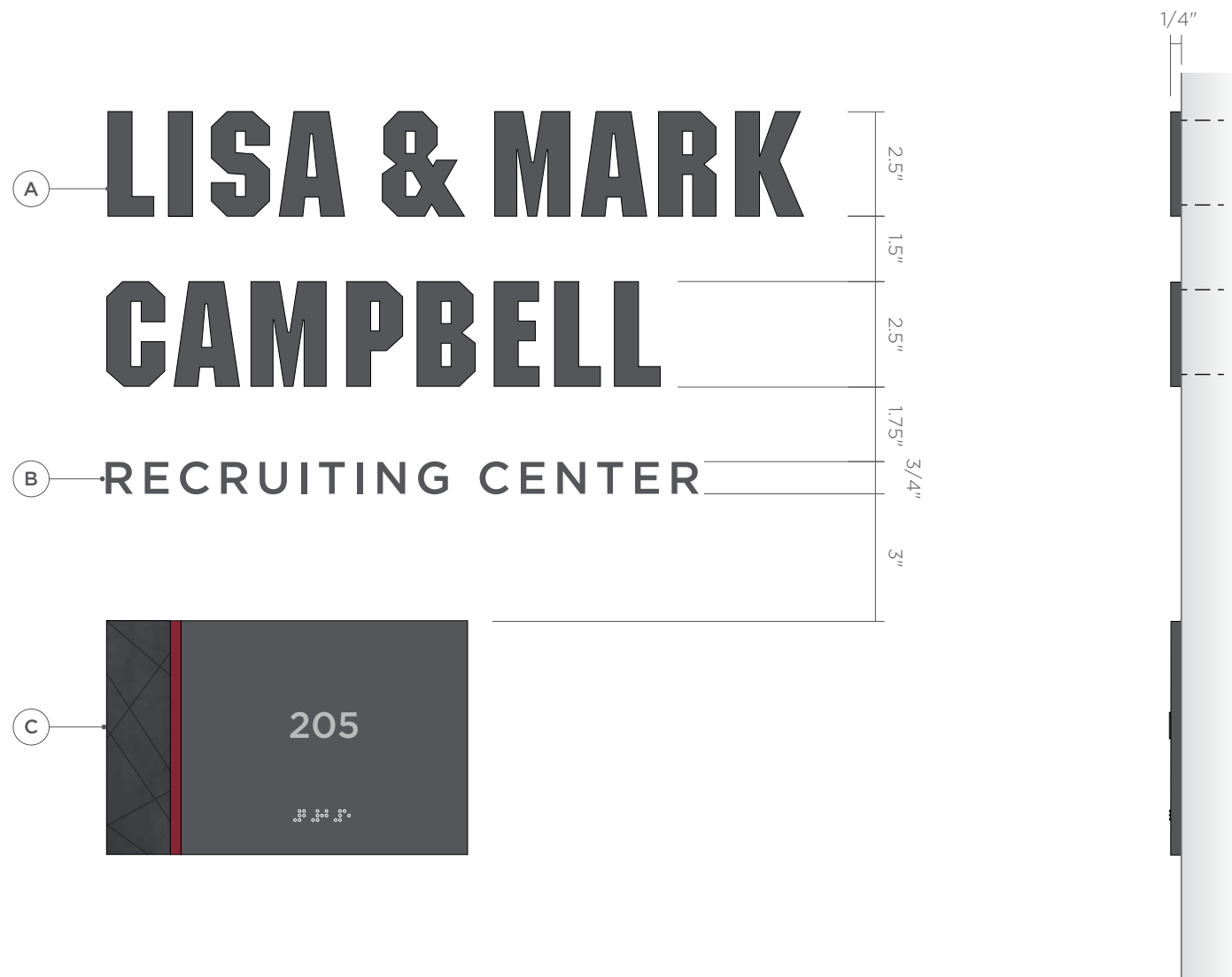
1 B1.1 - TYP. FRONT & SIDE ELEVATION SCALE: 3" = 1'-0"
