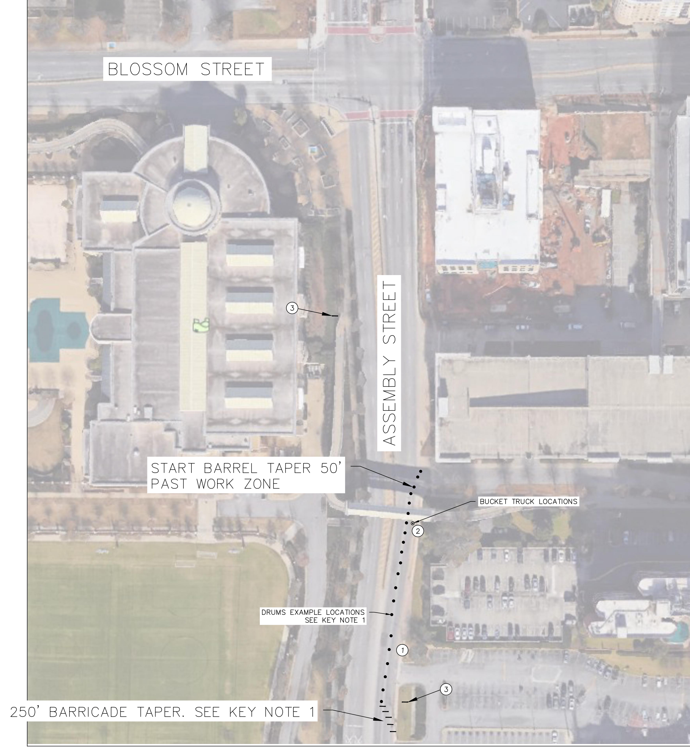
1 ASSEMBLY STREET PEDESTRIAN BRIDGE ROOF REPAIRS-TRAFFIC CONTROL STAGE 1 C1.2 NOT TO SCALE
