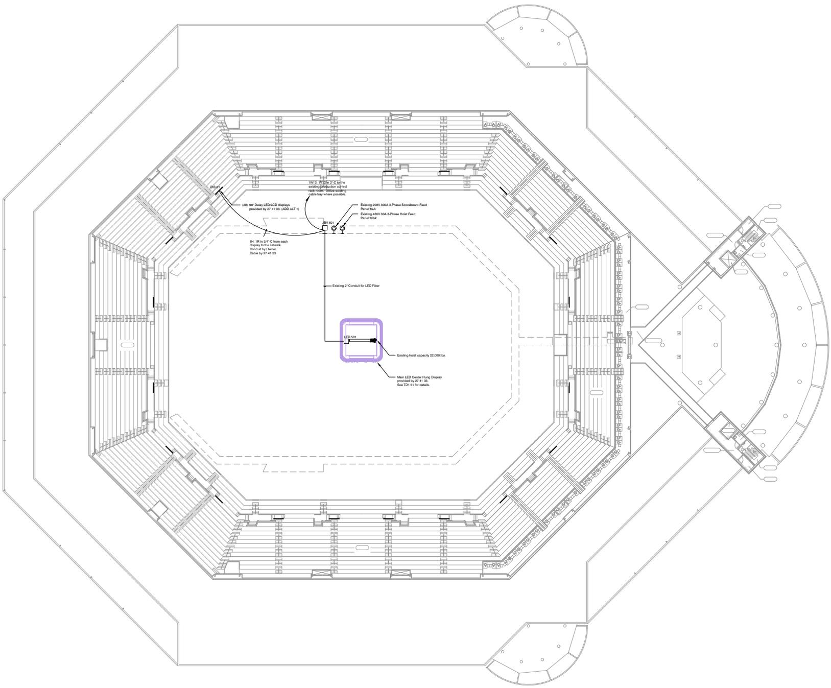
1W12, 1W120 2" C cable existing production control rack room - please existing cable tray where possible.
