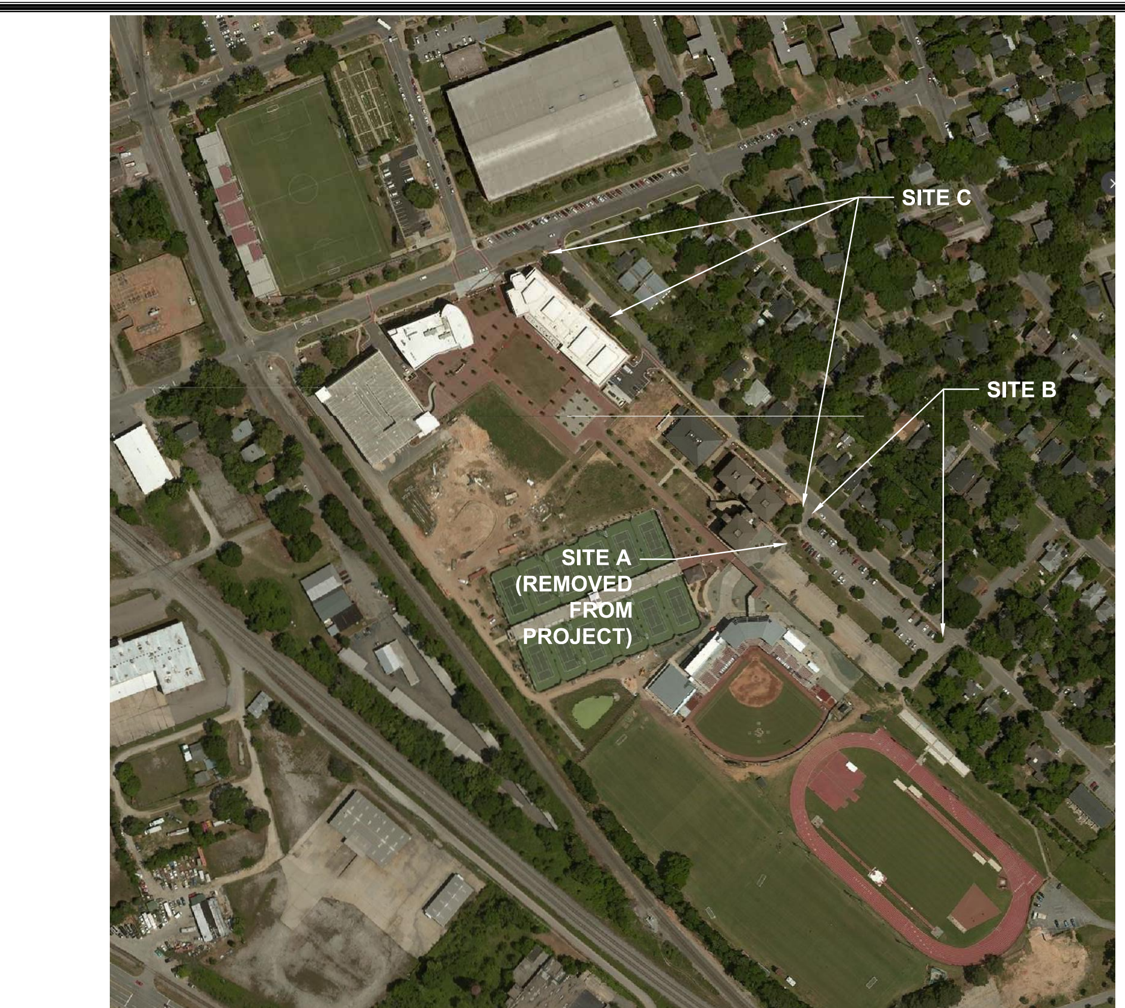
OVERALL SITE MAP SCALE: 1"=200' SITE A: REMOVED FROM PROJECT SITE B: SIDEWALK/CURB/LANDSCAPING REPAIRS ALONG SOUTH MARION STREET. SITE C: REPLACE SIDEWALK AND CURB SECTION. PAINT CURB ALONG SOUTH MARION STREET.
