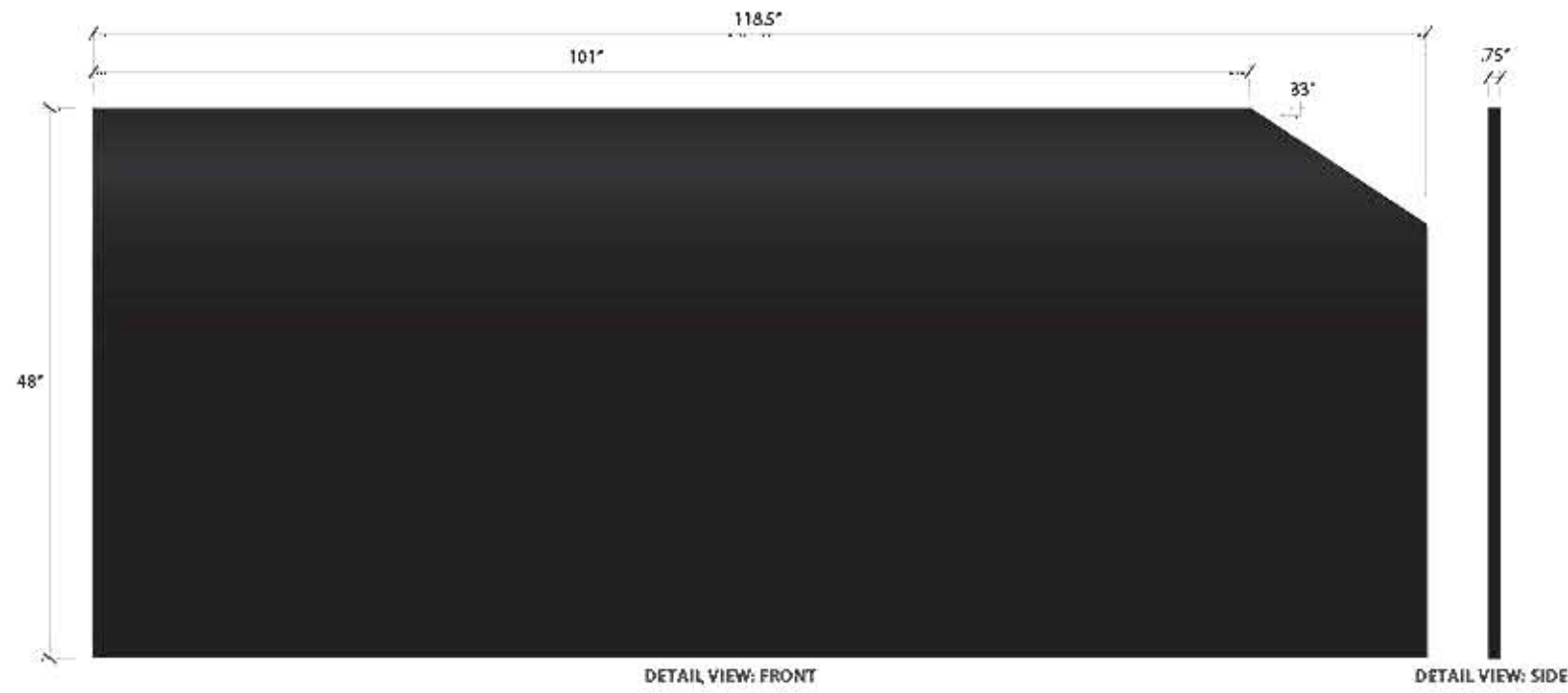
MELAMINE PANEL WITH GLOSS BLACK LAMINATE FACE AND SIDES - MOUNTS TO WALL WITH 'Z-CLIP' HANGER BAR SYSTEM
