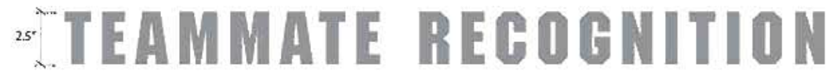
.25" THICK SINTRA WITH BRUSHED METAL FACE, SIDES PAINTED SILVER TO MATCH, APPLIED TO WOOD PANEL
