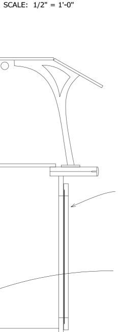
EXHAUST PANEL – CUSTOM PERFORATED INFILL PANEL SURROUNDED 4 SIDES BY 3/4" X 2" FRAME – PL 2 FACE & MATCHING PVC EDGES
