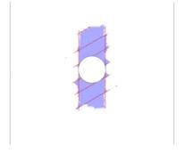
discontinuities associated with individual instances of matrix cracking occurring inside the composite plies, and delaminations at the interfaces between the plies. The DDM utilized Regularized eXtended Finite Element Methodology (Rx-FEM)[3].
