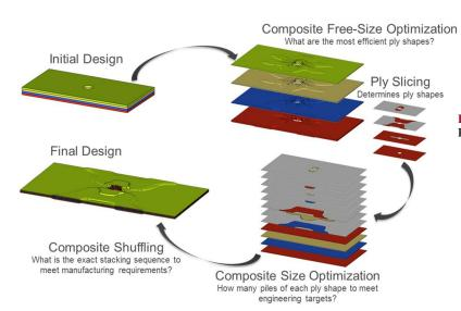
Figure 1. Results of 3-stage Composite Optimization Process Applied to an Open-Hole Tensile Coupon.
