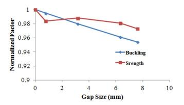
(3c). Predicted knockdown in strength and stability as function of gap size in stiffened composite panel subjected to shear loading.
