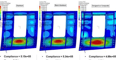
Figure 2. Results of 3-stage Composite Optimization Process Applied to an Aircraft Door Surround.
