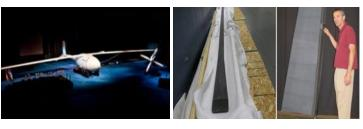
Figure 2. Phantom Eye thermoplastic AS4D/PEKK wing struts and T300/PPS rudder.
