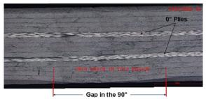
(1a). Micrograph of a composite laminate showing fiber waviness (top).
