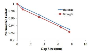
(3b). Predicted knockdown as function of gap size in strength and stability in stiffened composite panel subjected to axial compression loading.
