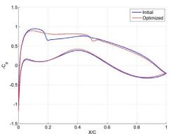
Figure 1. Pressure distribution at y/2b = 0.14 (top), 0.43 (second from top), 0.71 (second from bottom), 0.86 (bottom).
