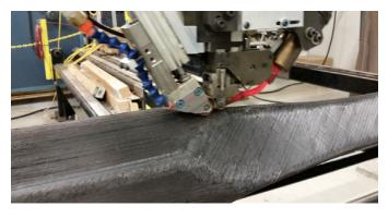
Figure 3. In-situ Automated Fiber Placement on an additive manufactured core.
