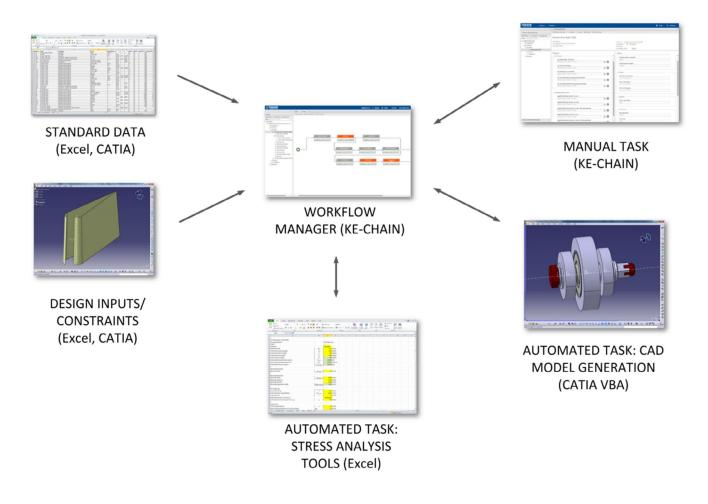
Figure 8. The Rudder-in-a-Month phase 1 main framework components, where the workflow manager orchestrates all data exchange and (automated) task execution.
