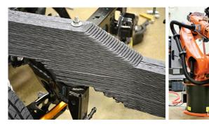
Figure 2. Extruded short fiber filled ABS frame of the ORNL BAAM Cobra car and robotic extruder.
