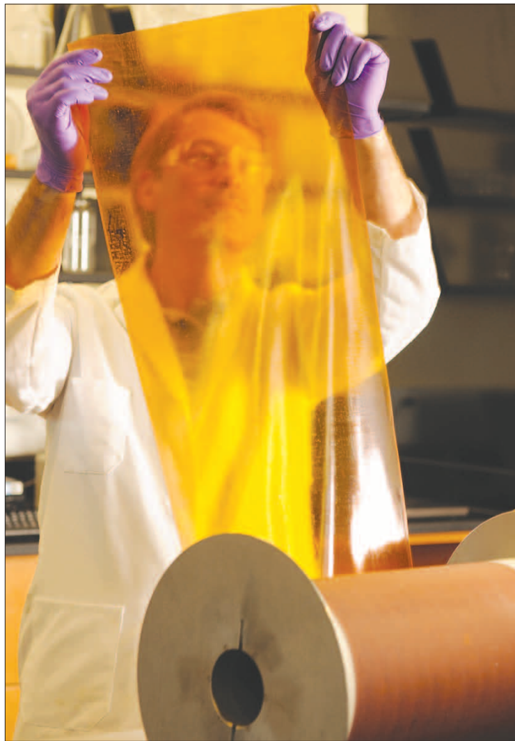
Heart of a fuel cell Brian Benicewicz, a Center of Economic Excellence professor, inspects a polymer membrane developed in his lab with assistance from industrial partner BASF. The polybenzimidazole membrane can operate at temperatures up to 200°C and is considered indispensable in creating silent, low-emission fuel cells used in back-up power systems for hospitals, telecommunications, and emergency centers.
