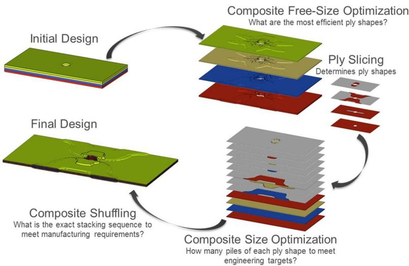
**Figure 1.** Results of 3-stage Composite Optimization Process Applied to an Open-Hole Tensile Coupon.
