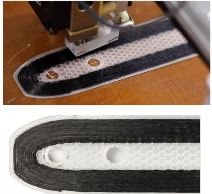
Figure 1. MarkForged carbon/PA tension strap.
