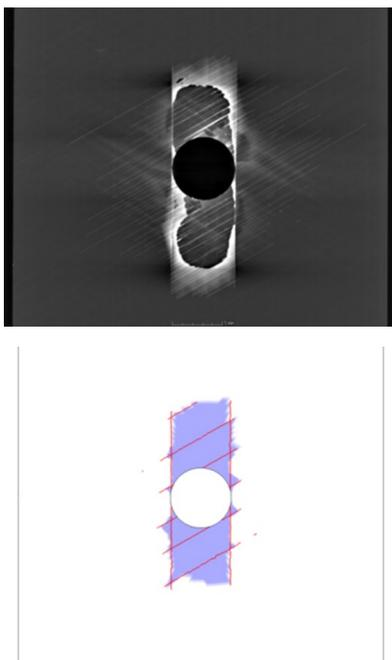
discontinuities associated with individual instances of matrix cracking occurring inside the composite plies, and delaminations at the interfaces between the plies. The DDM utilized Regularized eXtended Finite Element Methodology (Rx-FEM)[3].
