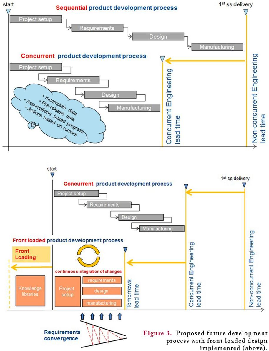
**Figure 3.** Proposed future development process with front loaded design implemented (above).
