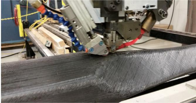
**Figure 3.** In-situ Automated Fiber Placement on an additive manufactured core.
