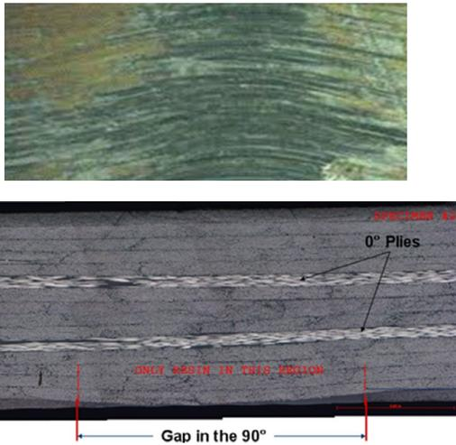
(1a). Micrograph of a composite laminate showing fiber waviness (top).
