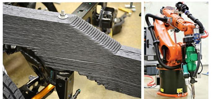
Figure 2. Extruded short fiber filled ABS frame of the ORNL BAAM Cobra car and robotic extruder.
