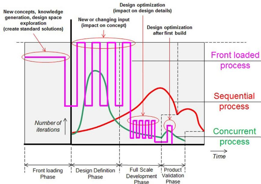
Figure 4. Iterations sequential, concurrent and front loaded development process for new design-build.
