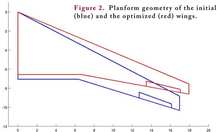
Figure 2. Planform geometry of the initial (blue) and the optimized (red) wings.
