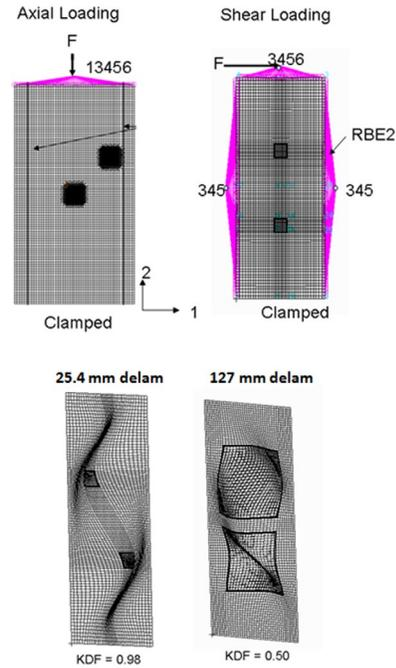
(2a). Finite element models for axial compression and shear buckling with initial delamination (top).
