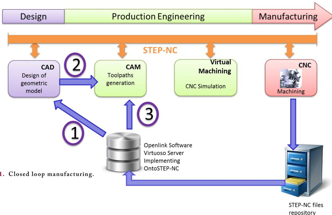
Figure 1. Closed loop manufacturing.
