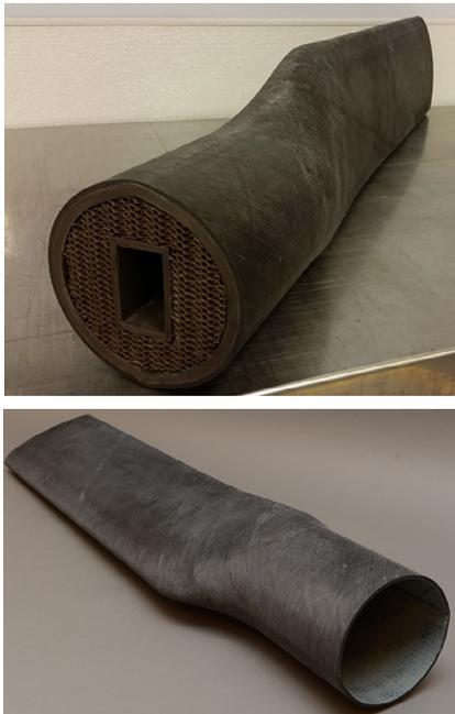
**Figure 4.** Additively manufactured advanced composite structure before (top) and after (bottom) core is washed out.
