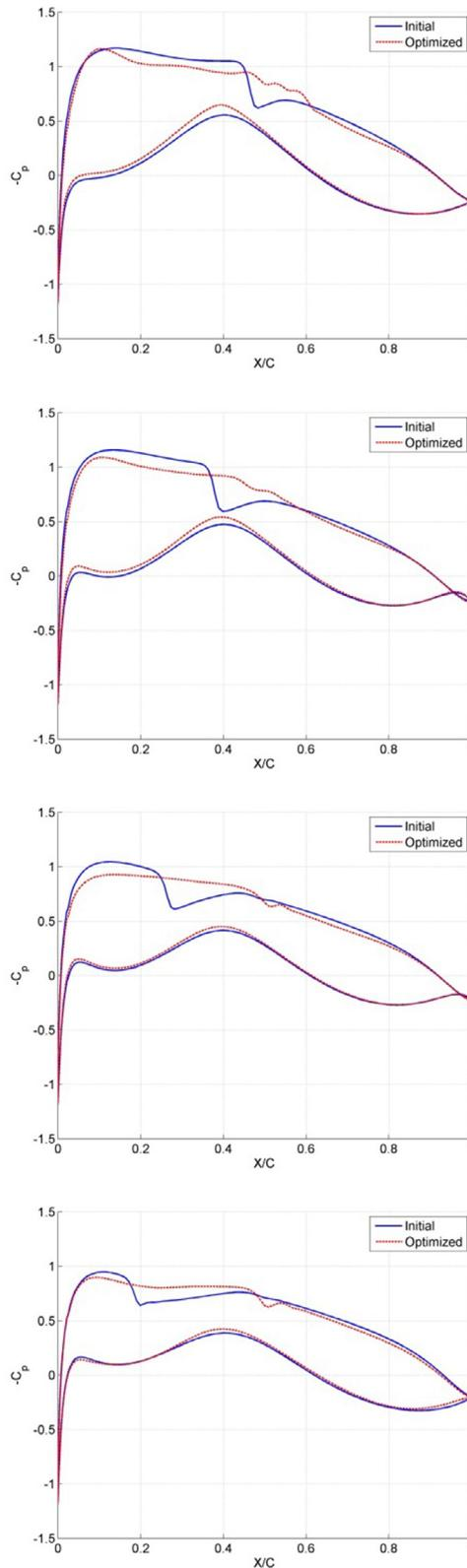
Figure 1. Pressure distribution at  $y/2b = 0.14$  (top),  $0.43$  (second from top),  $0.71$  (second from bottom),  $0.86$  (bottom).
